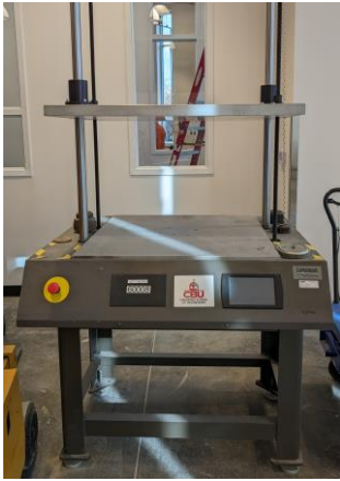
Lansmont Squeezer Compression Table (5000-lb capacity)
