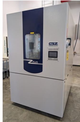
CSZ ZPH-64-2-H/AC Z-Plus Temperature & Humidity (64 CF test space volume, -30F to + 375F temperature range, 10% to 98% RH range)
