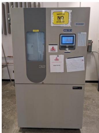
CSZ Temperature & Humidity Chamber Model ZP-32 (-49F to +374F, 10% to 98% RH, 38"x38"x38" chamber size)
